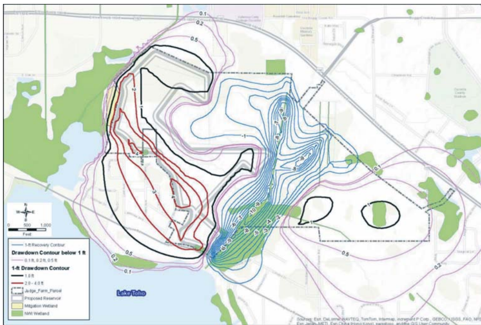
Figure 4. Projected Average Drawdown in Wetland Water Levels for Alternative With Judge Farms Reservoir at 51 ft NGVD and Local Soils K_h = 2 ft/d
